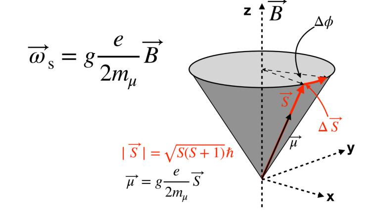
The anomalous spin precession frequency  $\overrightarrow{\omega}_a = \overrightarrow{\omega}_s - \overrightarrow{\omega}_c$
