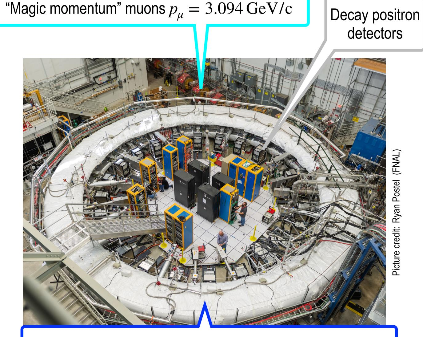
14-m diameter superconducting magnet with high-precision vertical B=1.45 T field
